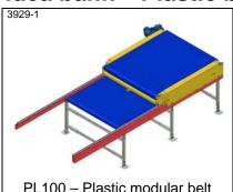
PL100 - Plastic modular belt conveyor with telescopic extension, retracted
