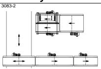
PL1500 – Plastic modular belt conv. Trays, side by side, are arranged in a row on transfer car
