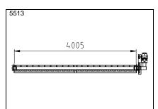
PL1500 – Plastic modular belt conveyor. Cooling conveyor, 4 m wide, 25 m long
