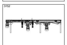
PL100 - Plastic modular belt conveyor with small radius idler rollers and pneumatical stops
