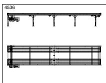
PL100 - Plastic modular belt conveyor, 2-strings with small radius idler rollers
