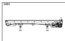
PL1500 - Plastic modular belt conveyor with small radius idler rollers, end mounted motor
