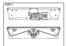
PL1500 - Plastic belt conveyor with centre and small radius idler rollers
