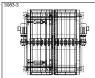
PL1500 – Plastic modular belt conveyor. Parallel conveyors of which one is movable sideways.
