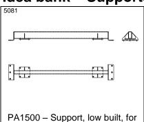
PA1500 - Support, low built, for mounting of conveyor on load cells
