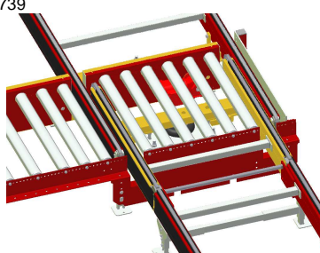
PA1500 – Tiltable chain conveyors coming into roller conv. from opposite directions
