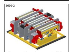
KE500 - Transfer car with lifting and lowering roller conv. With chain conv. through both sides
