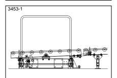
PA1500 - Transfer car, undriven. Tilting of conveyor and stop in conveyor foot operated
