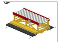
PA1500 - Transfer car. Sturdy for heavy loads, up to 3600 kg. Equipped with bumpers
