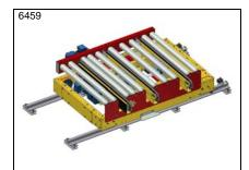
PA1500 – Transfer car with roller conv. with transveyor. Running on rails. With guide wheels
