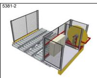
PA1500 – Transfer car with 4 conveyors and platform. 3 conveyors sideways moveable
