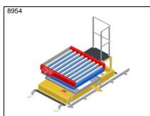
PA1500 - Transfer car with roller conveyor on lift table and platform for operator
