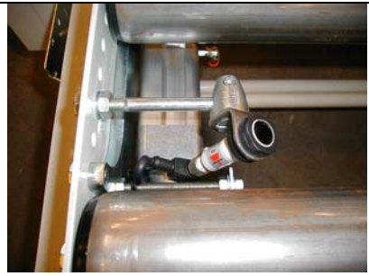
Bracket for M18 sensor.
